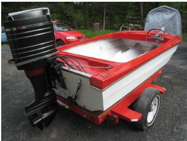
Power trim wasn't available till 1967, but Mercury published a guide for installing the later model trim on the earlier Mercury outboards. It took a while, but came together with parts from a number of sources.
