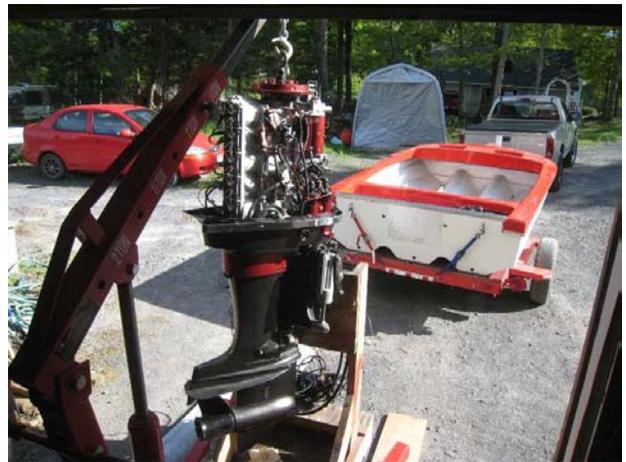
With the deck attached to the hull now inside and out, it was time to install the outboard and power trim/tilt that had been adapted to the motor.
