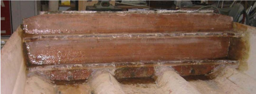
Next was sanding and then painting the interior. This is actually a two part epoxy coating. As can be seen clearly here, the hull is the floor. Watch your step!
