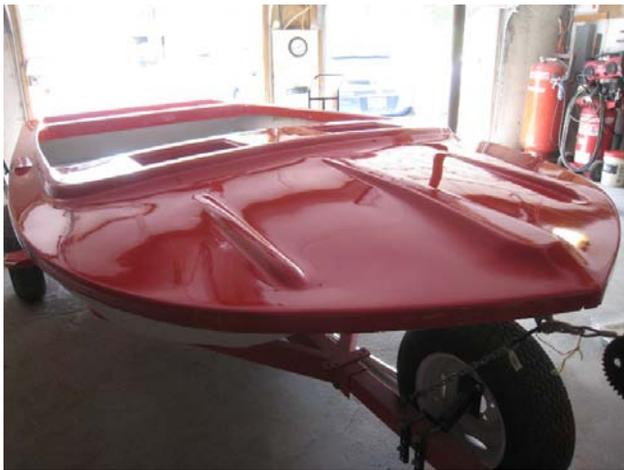
In early 2010 the deck was done and ready for rub rail and fiberglassing of the seam between the deck and hull. We glassed a 3" strip in first, then a 6" strip overtop of it. We didn't get all the way to the bow peak (it's a bit tight in there), but we got most of the way.
