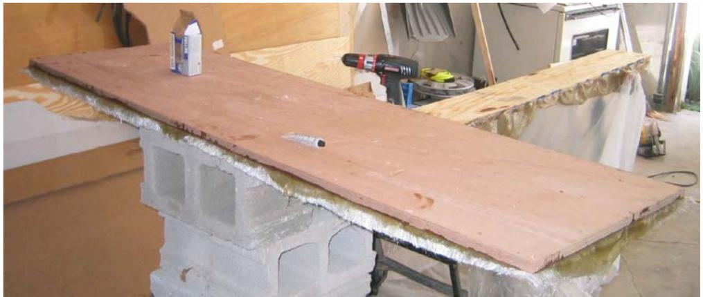
Work progressed. The newly made transom core was fiberglassed in with two cross braces. The original Power Cat had one cross brace, but I wanted a rock strong transom. It was glassed in overlaps tying it to the sides of the hull as well as the floor.
