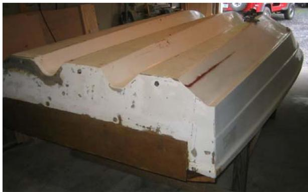
With that done, the hull could be flipped for work on the exterior. There were substantial gel coat cracks all over it.
