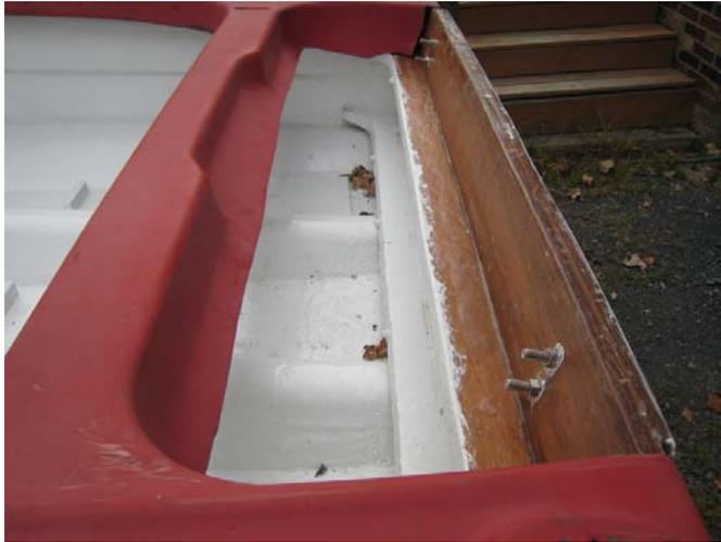
Once the deck was on, it was time to carefully trim the old splash pan out to construct a new one for the taller transom. The top crossmember had been placed in part to be a rest for the 1/4" luan plywood base for the new splashpan. Doing this also securely tied the rear of the deck to the hull.
