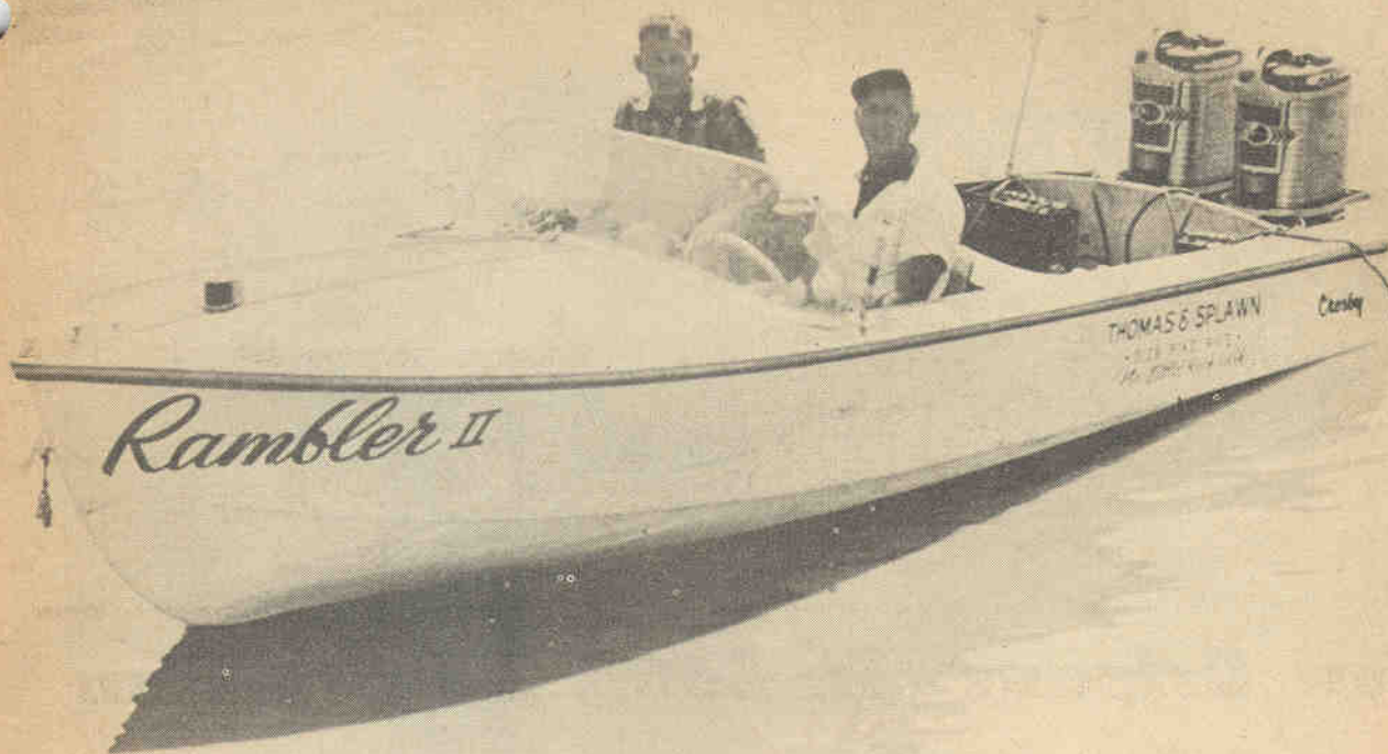
Lyndon Graham, left, and Roy Cullum, author of this article, shared the driving on the 1053-mile dash. Boat is twin Mercury Mark 75-powered Crosby.
