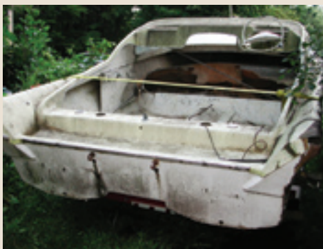
Moss never sleeps...the Power Cat is looking pretty funky after years of neglect during outside storage. View of the shattered transom and missing starboard fin. Molded fiberglass fuel tanks under the splash well—the water pump installed through the floor. After a thorough cleaning, the inside, amazingly, was in near-to-perfect condition. Shot of the manufacturer's plate.
